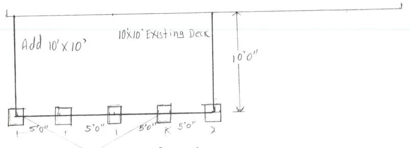
Brick Piers on a 18" x 18" sq x 8" Thick Poured Conc. Footing.
