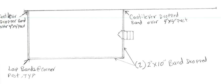
1st Floor framing plan.
