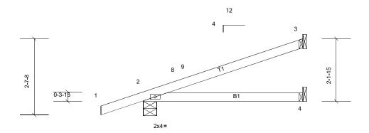
Scale = 1:28.2 Loading (psf) **Spacing** 2-0-0 CSI **DEFL** (loc) I/defl L/d **PLATES GRIP** TCLL (roof) 20.0 Plate Grip DOL 1.15 TC 0.30 Vert(LL) 0.03 4-7 >999 240 MT20 244/190 **TCDL** 10.0 Lumber DOL 1.15 BC 0.23 Vert(CT) -0.07 >909 180 4-7 **BCLL** 0.0 Rep Stress Incr YES WB 0.00 Horz(CT) 0.00 2 n/a n/a **BCDL** IBC2015/TPI2014 FT = 20% 10.0 Code Matrix-MP Weight: 19 lb
