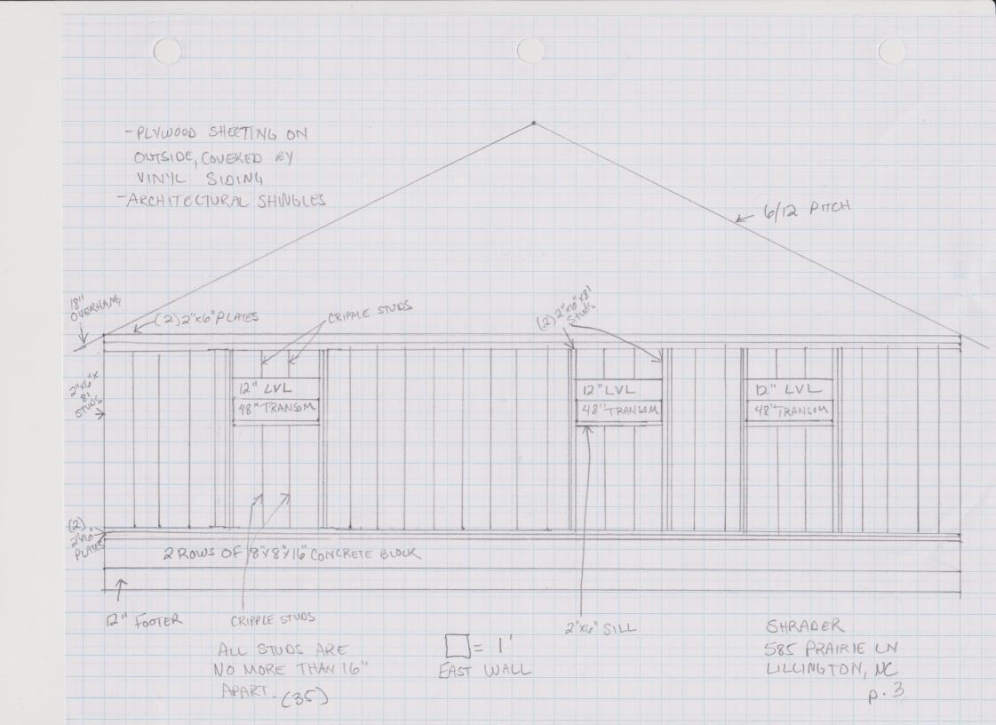
SIDE VIEW OF OUTSIDE WALL W/FOOTERS (2) 2"x 6" PLATES - 1/2" REBAR ANCHOR STANDARO 12 Inches wide 8 x 8 x 16" minimum code if CONCRETE BLOCK mono. 16 wide minimum if stemwall. SHOP FLOOR 1/2 REBAR ANCHOR 4" CONCRETE W/3/8" REBAR WIREMESH 12" CONCRETE VAPOR RETARDER FOOTER ]=2" 3-4" Waster > STONE SHRADER (#57 or 67) 585 ARAIRIE LN LILLINGTON, NC \* AUTUST THESE "WIDE
