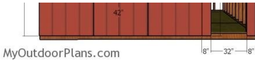
Side wall siding sheets
