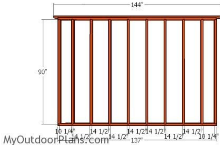
Back wall frame
