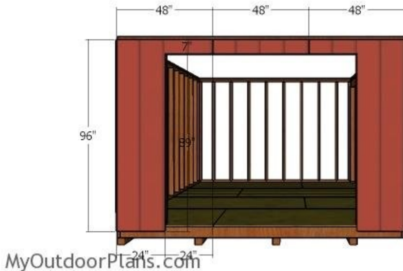
Front siding sheets
