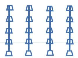
Shed mounted on 20 pier blocks 4x4's running across pier blocks Gravel over entire area on the ground to facilitate drainage
