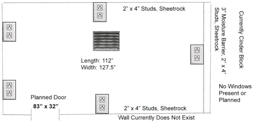
Construction: Cover Existing Cinder Block Wall, with Moisture Barrier, Insulation, Wall, and Sheetrock; Build Interior Walls; Incorporate Door Frame; Electrical: Install (5) Outlets; HVAC: Incorporate (1) Register
