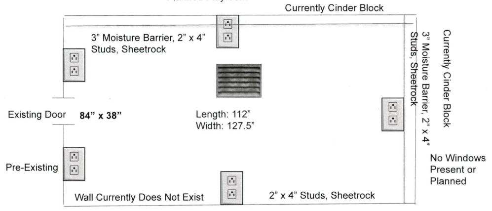
Construction: Cover Existing Cinder Block Walls, with Moisture Barrier, Insulation, Wall, and Sheetrock; Build Interior Wall; Electrical: Install (4) Outlets; HVAC: Incorporate (1) Register
