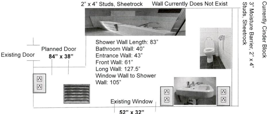
Construction: Cover Existing Cinder Block Wall, with Moisture Barrier, Insulation, Wall, and Sheetrock; Build Interior Wall; Electrical: Install (3) Outlets; HVAC: Incorporate (1) Register
