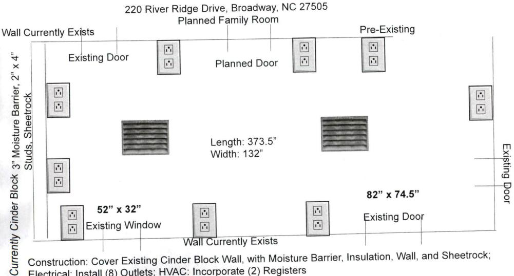
Construction: Cover Existing Cinder Block Wall, with Moisture Barrier, Insulation, Wall, and Sheetrock; Electrical: Install (8) Outlets; HVAC: Incorporate (2) Registers
