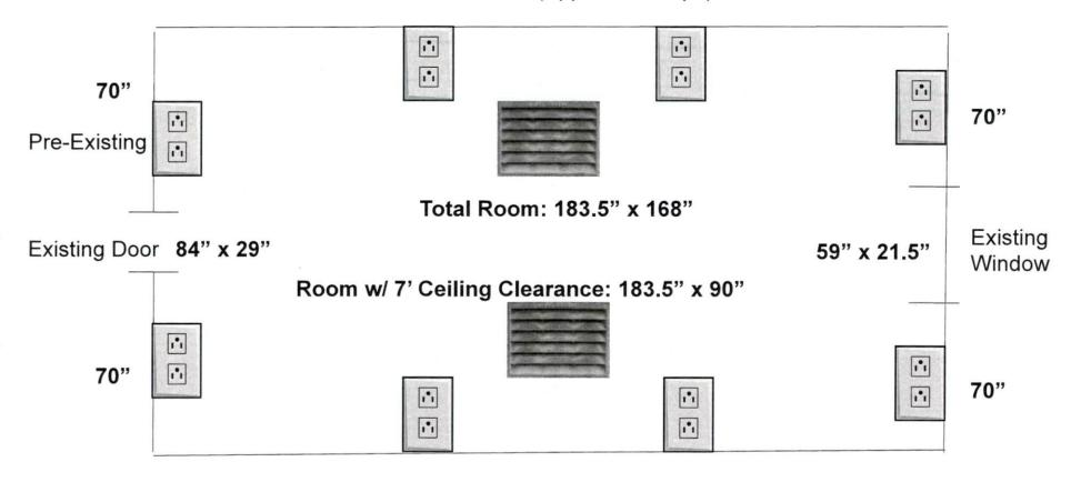
Construction: Install Insulation and Sheetrock; Electrical: Install (7) Outlets; HVAC: Incorporate (2) Registers
