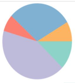
4,651.2 BTUh Windows, glass doors, skylights: 16,167.6 BTUh Envelope (walls, doors, roof, etc.): Infiltration: 2,765.7 BTUh 11,415.1 BTUh Duct heat loss: Ventilation/winter humidification: 3,225.8 BTUh Hot water piping load: 0.0 BTUh Total heating: 38,225.4 BTUh
