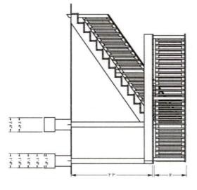
DISCLAIMER: ONLY USE #2 OR BETTER PRESSURE TREATED SOUTHERN PINE 2X10 FOR FRAMING MATERIALS. NEVER SUBSTITUTE SOFTWOODS OR COMPOSITE FOR FRAMING MATERIALS.
