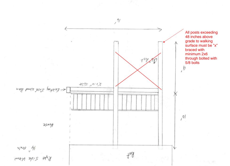
Front View of Front Porch 14 scale 10, 0 Minimum 2x8 @ 16" oc ceiling joists Collar Ties every third rafter 2x10" Floor Joist Rafters at 16" oc
