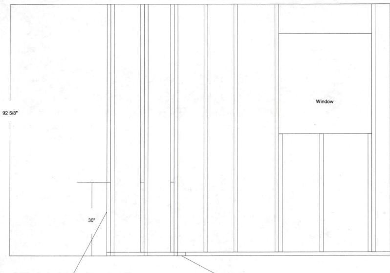
Cut 30" section from 3 exterior wall studs and scab 30" section with #2- 2" X 4" and a full length stud sistered next to it.
