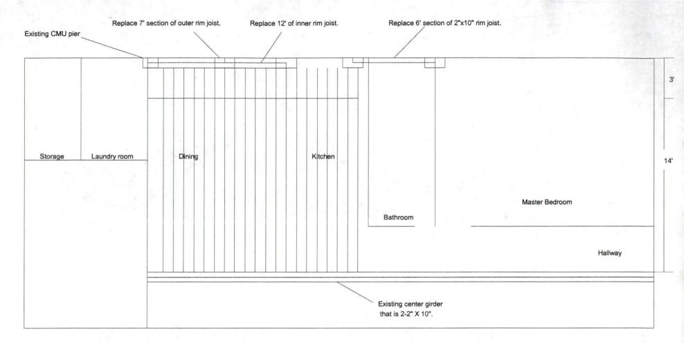
Lumber used to replace rim joist will be presure treated 2" x 10" #2 lumber.
