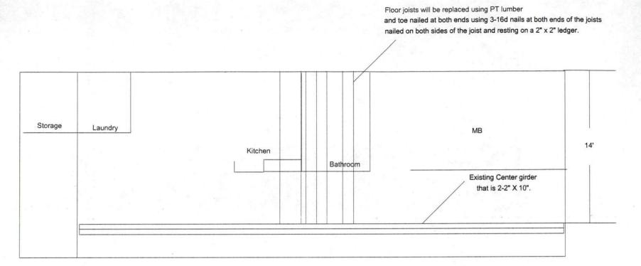
Lower wall plate will be replaced using 2" x 4" studs .
