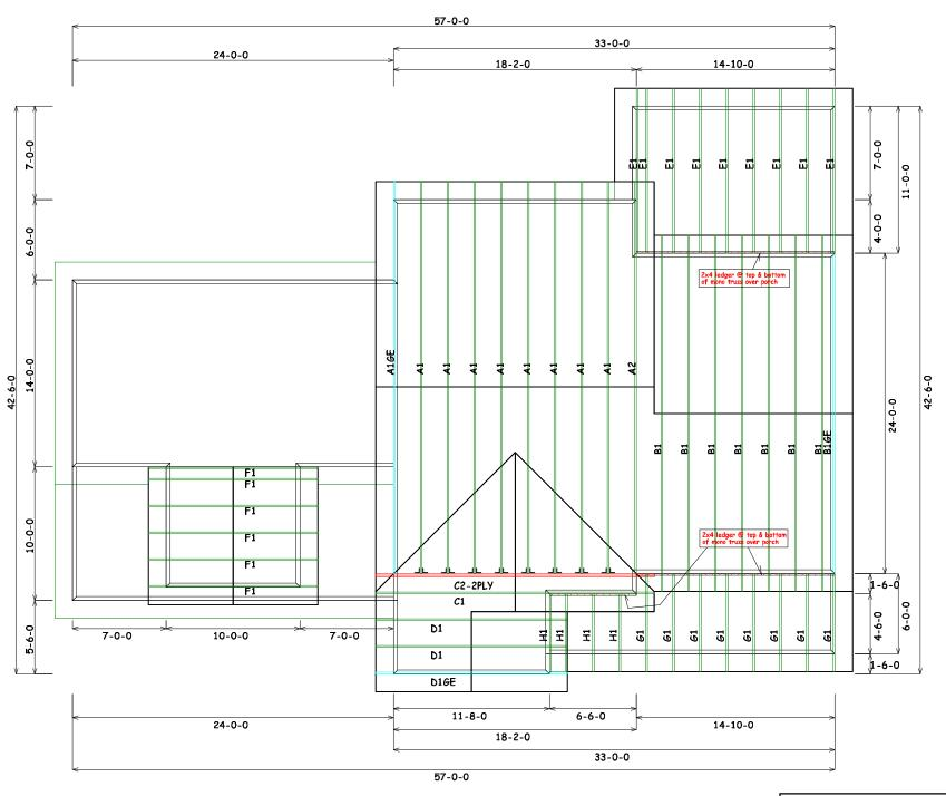
⊔ = Simpson HUS28 / hanger Use Simpson H2.5 Ties on all bearings, except truss A2 use (2) H2.5's at joint #19, truss C2-2PLY use Simpson LGT2 at each bearing.
