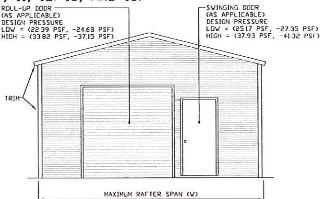
TYPICAL END ELEVATION-HORIZONTAL ROOF SCALE: NTS
