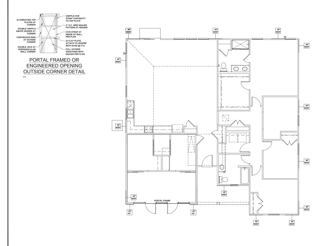
FIRST FLOOR WALL BRACING PLAN - 'L'
