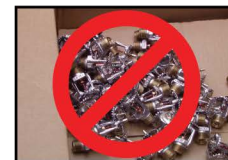
INCORRECT (Stored loose in a box)
