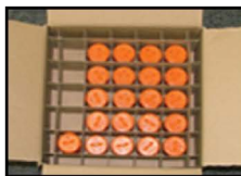
CORRECT (Protective caps in place)
