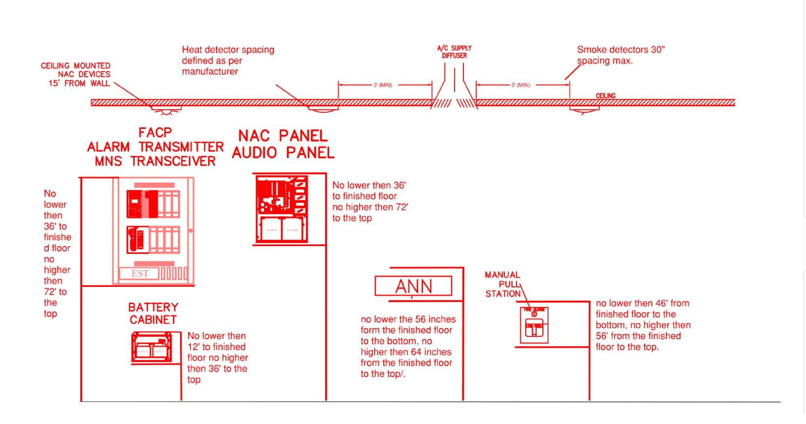
All FA equipment as FACU and BPS-APS or battery boxes shall be installed using toggle bolts with washers.
