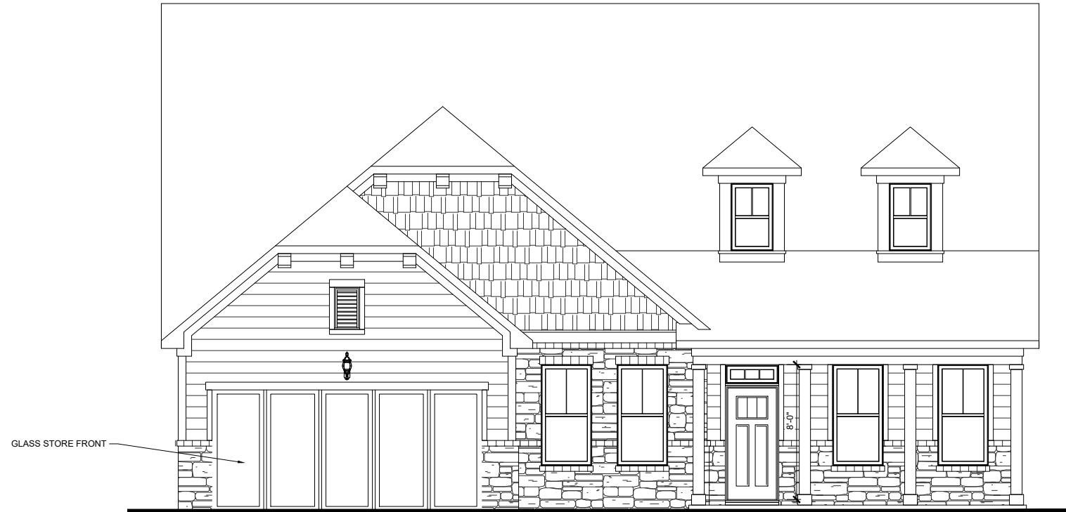
FRONT ELEVATION - 'B' SCALE: 1/8"=1'-0" (11"X17" SHEET SIZE) SCALE: 1/4"=1'-0" (22"X34" SHEET SIZE)
