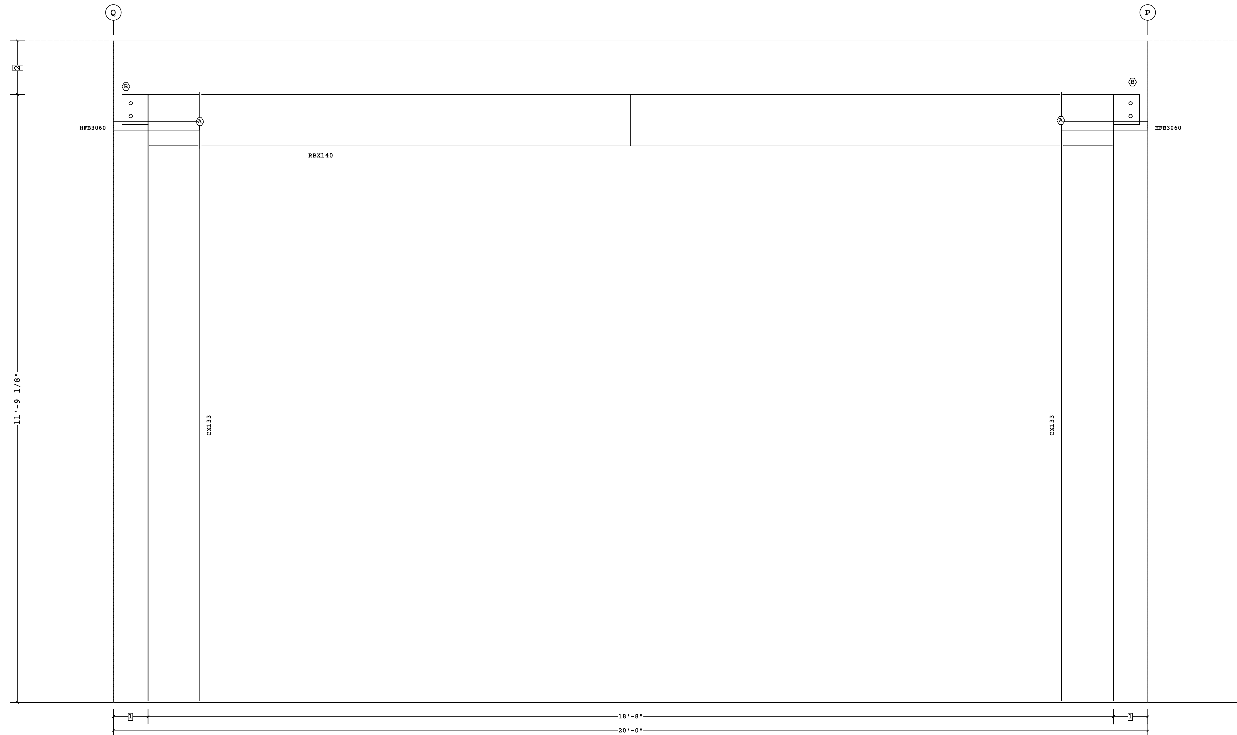
PORTAL FRAME ELEVATION ALONG 7
