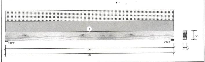
Reactions UNPATTERNED lb (Uplift) Member Information Wind Live Dead Snow Application: Floor Direction Type: Girden 3933 3510 0 0 Plies: 4 Design Method: ASD 1 Vertical Building Code: IBC 2018 0 3933 3510 0 Moisture Condition: Dry 2 Vertical Load Sharing: Deflection LL: 360 Yes Deflection TL: 240 Deck: Not Checked Importance: Normal - II Temp <= 100°F Temperature: Bearings General Load Ld. Comb. Cap. React D/L lb Total Ld. Case
