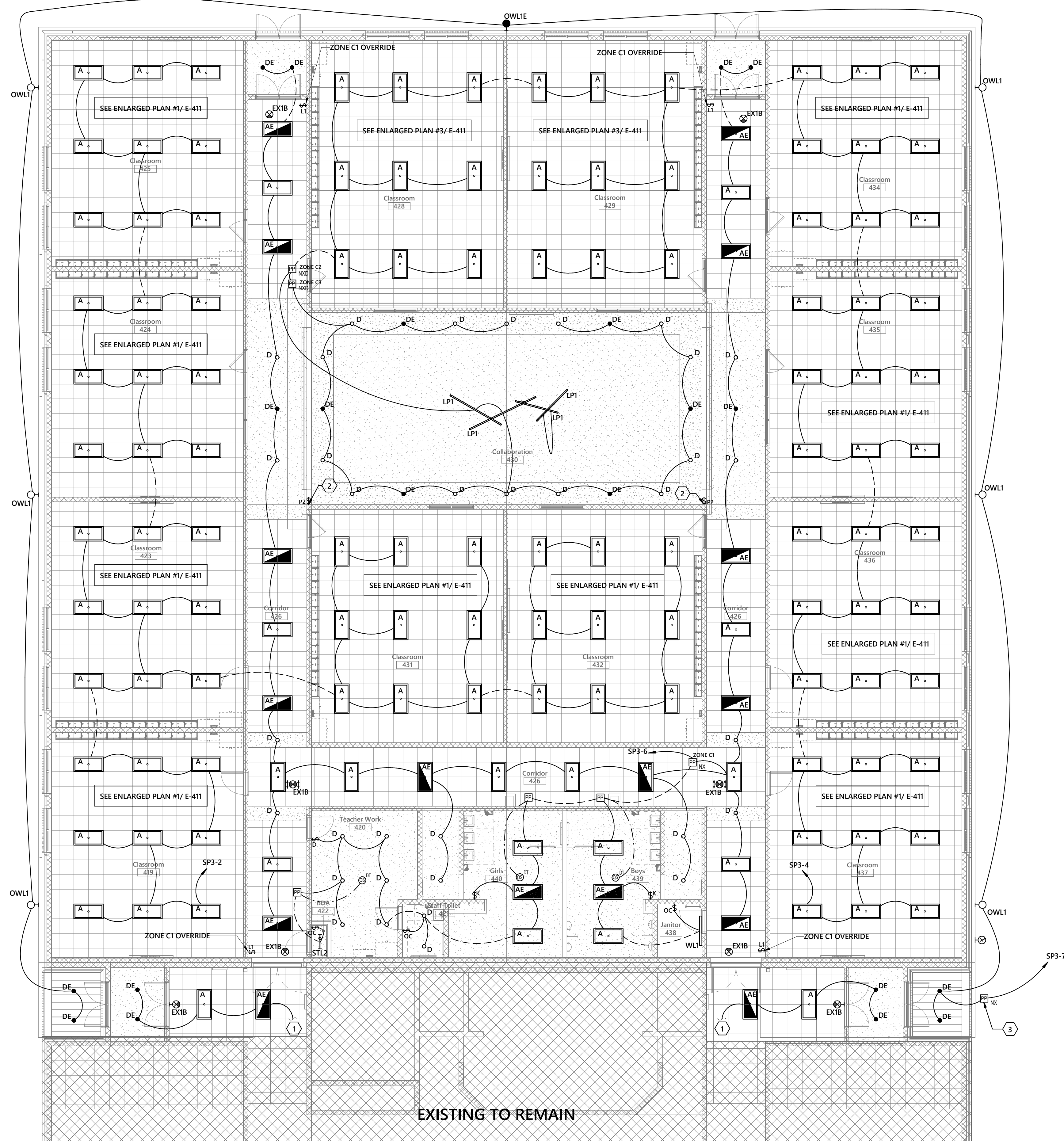
1 CLASSROOM ADDITION LIGHTING PLAN - NEW WORK 1/8" = 1'-0"
