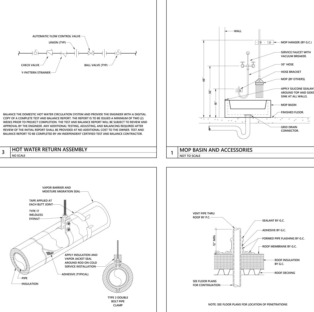
VENT THRU ROOF DETAIL
