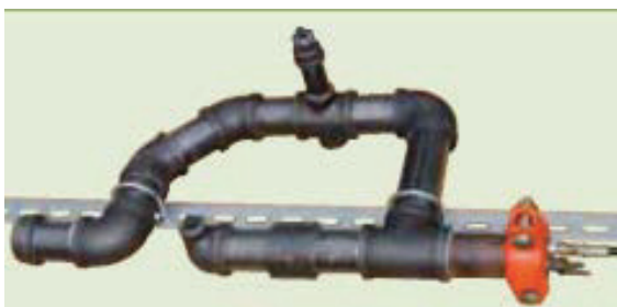
Burst pressure testing of DI threaded fittings (2”)
