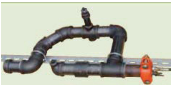
Burst pressure testing of DI threaded fittings (2")
