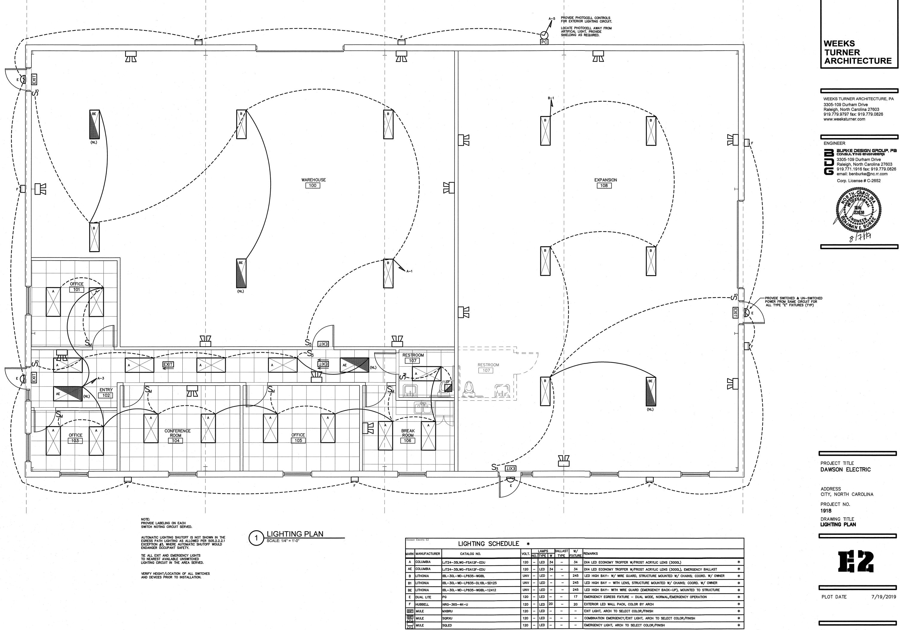
OR APPROVED EQUAL. PROVIDE CUT SHEETS FOR OWNER APPROVAL PRIOR TO ORDERING FIXTURES. FOR FLUORESCENT FIXTURES CONTROLLED BY MOTION SENSOR, PROVIDE "PROGRAMMED RAPID START" BALLASTS. CATALOG NUMBERS ARE FOR REFERENCE ONLY, ACTUAL NUMBERS MAY VARY. 'EB' DENOTES ELECTRONIC BALLAST. VERIFY FIXTURE HAS INTEGRAL LOCAL DISCONNECTING MEANS PER NEC 410.130 (G).
