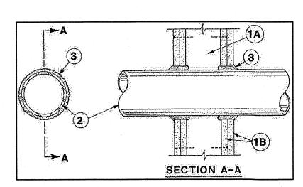
1. Wall Assembly -- The 1, 2, 3 or 4 hr fire-rated gypsum wallboard/stud wall assembly shall be constructed of the materials and in the manner described in the individual U300 or U400 Series Wall or Partition Designs in the UL Fire Resistance Directory and shall include the following construction features:
