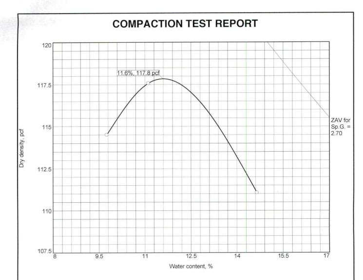
Test specification: ASTM D 698-07 Method A Standard
