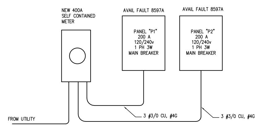
AVAIL FAULT 8597A 50 KVA OH TRANSFORMER 2%Z 100'-0" TRIPLEX
